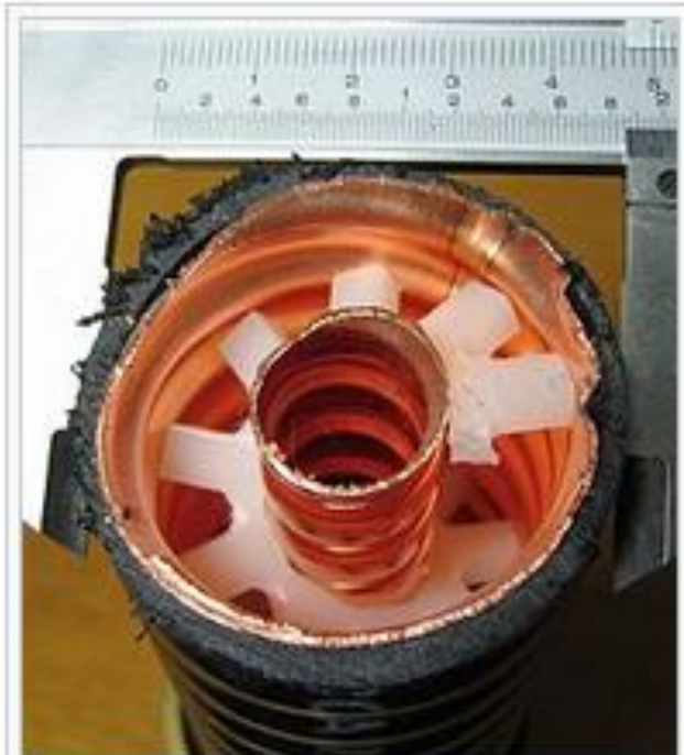
1 \frac{5}{8} in (41 mm) flexible line with (mostly) air dielectric
